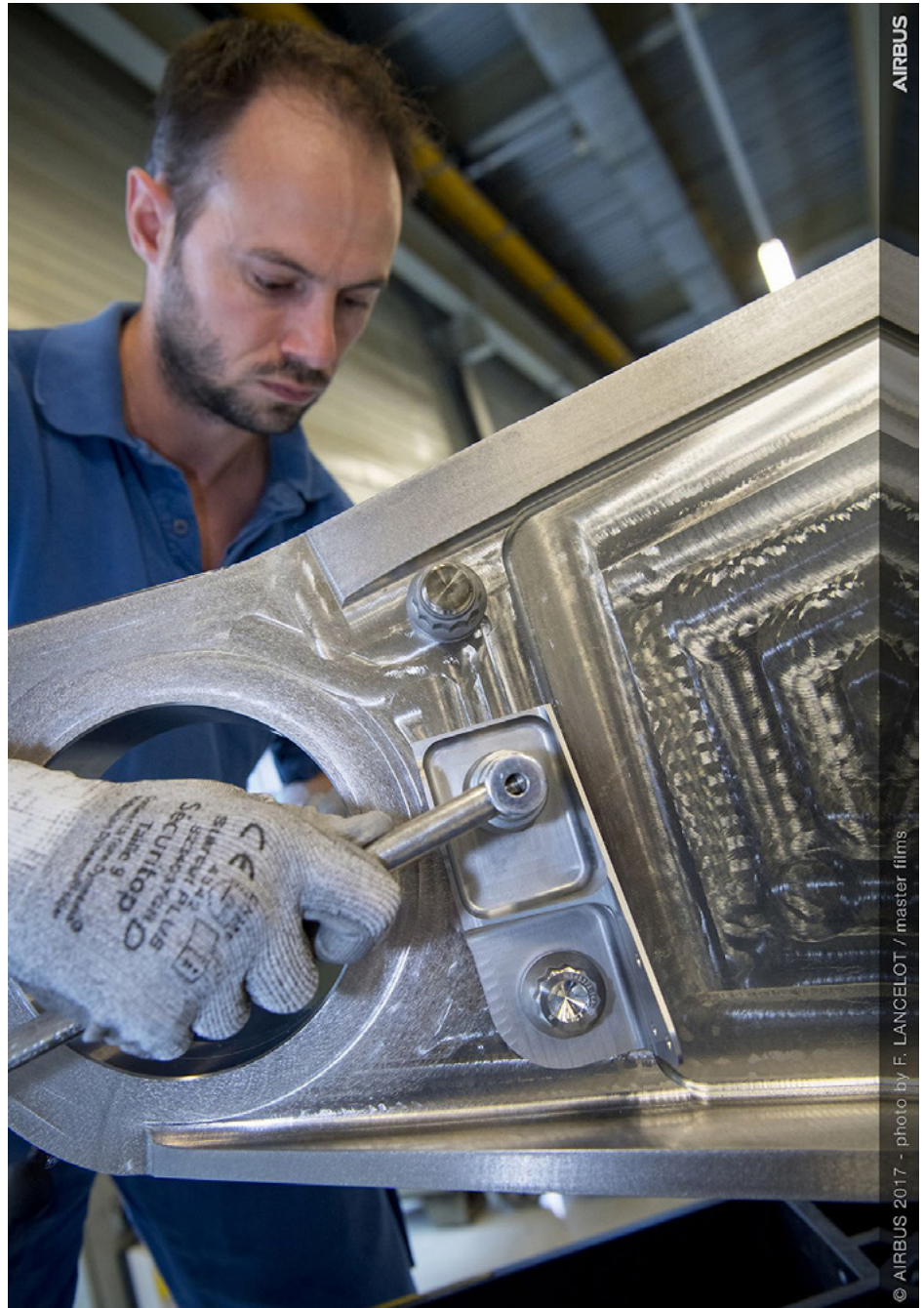
Arconic and Airbus achieve a 3D printing first—the installation of a 3D printed titanium bracket, shown here, onto a series production Airbus commercial aircraft, the A350 XWB.
